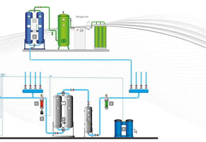
**5. Condensate drain:** Drains are needed at all separators, filters, dryers and receivers in order to remove the liquid condensate from the compressed air system.
