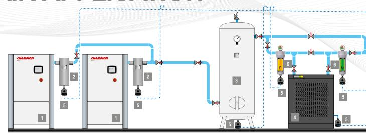
**1. Compressor:** The basic working principle of an air compressor is to compress atmospheric air, which is then used as per the requirements. In the process, atmospheric air is drawn in through an intake valve; more and more air is pulled inside a limited space mechanically by means of piston, impeller, or vane.
